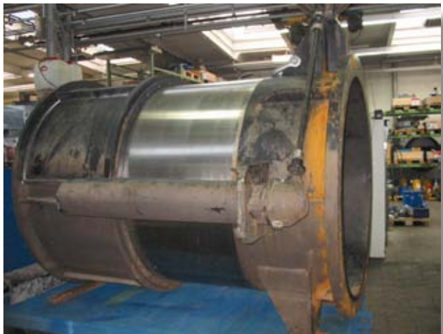
Disassembly of the 10-year-old VAG KSS Hollow Jet Discharge Valve
