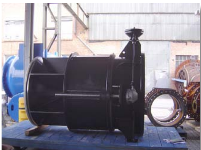
VAG KSS Hollow Jet Discharge Valves after rehabilitation
