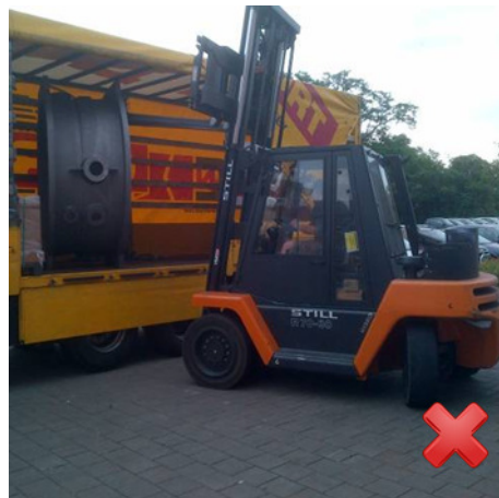
Negative example: unloading from one side not possible
