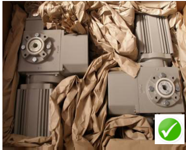
Safeguarding of packing pieces against damage by means of filling material
