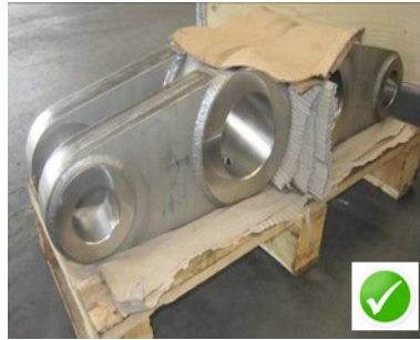
Safeguarding of packing pieces against damage by means of filling material
